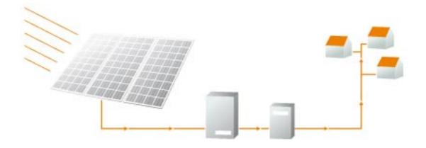
Functional principle of a photovoltaic plant
